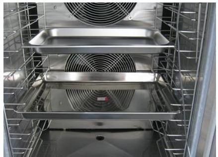
For quick cooling, sheet metal or foil containers with high thermal conductivity should be used. Plastic or polyurethane containers isolate the food from cool air. When cooling non-fractional food, the use of proper gastronomic or similar containers is recommended.
