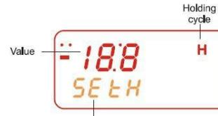
In this exemplum the set point of the holding cycle is modified.
