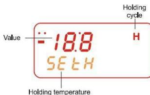
In this exemplum the set point of the holding cycle is modified.
