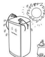
Is the location exposed to direct sunlight or too close to the furnace and other heat sources
