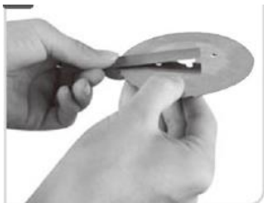
Remove any burrs from the cutting edge on the top side.
