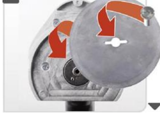
7. Install the new blade. Screw on the pressure disk and the screw.
