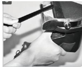
Carefully remove any burrs on the top side of the blade.
