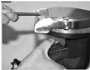
Sharpen the toothless blade for about 1...2 seconds at a low angle on the underside.
