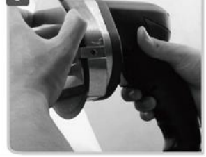
8. Reattach the blade guard and locking screw.
