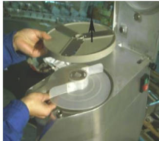
Installation of the cutting plate (4)
