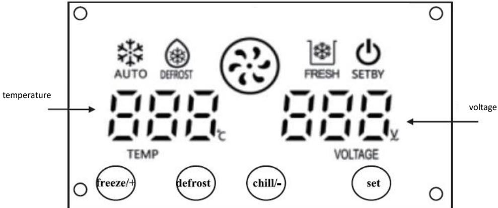
5.1 When the power is on, the SETBY LED lights up. The left side of the display shows the temperature, the right side shows the voltage.
