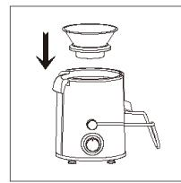
3. Close the bowl with the lid (3) so that the lid's discharge opening is directly above the waste container.
